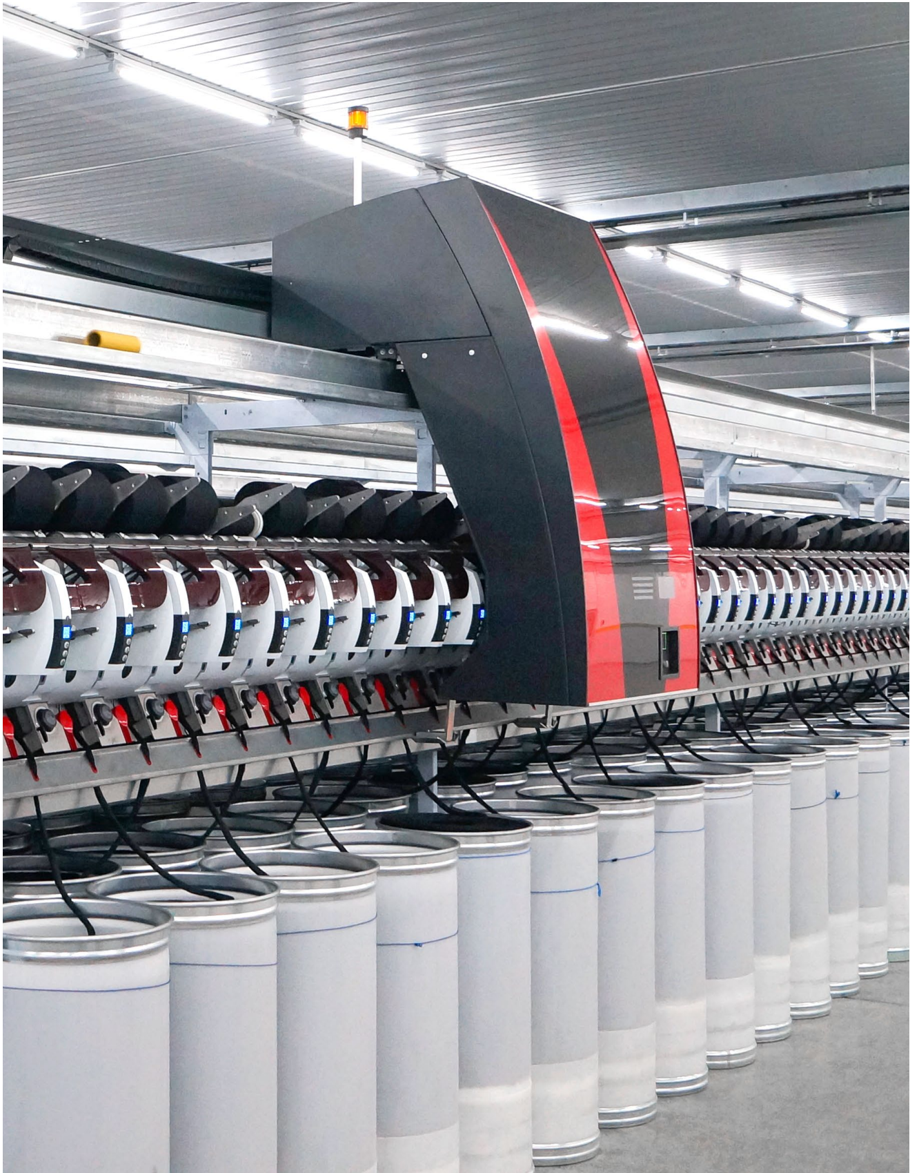
The fully automatic rotor-spinning machine Autocoro is an asset to customers who want to produce sustainable yarns from recycled products.
