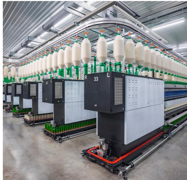
The Autoflow rails allow the roving bobbins to be transported interruption-free. Autoflow makes your production successful through the intelligent control, low-maintenance and well thought out components, and your downtimes are reduced significantly.
